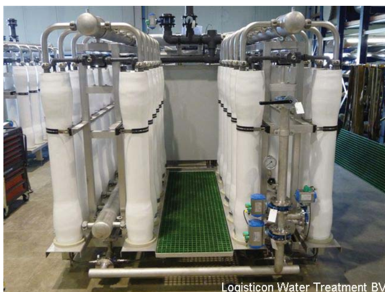
Fig. 1.6. Full scale RO installation with the first spiral wound membrane modules placed vertically for two-phase flow cleaning application for fouling removal in Botlek area, Rotterdam, the Netherlands (picture courtesy of Logisticon).
